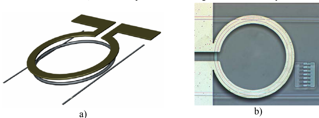
Figure 6.2. Isometric rendering a) and a realized version b) of a vertically coupled MR building block that has side-coupled port waveguides. The marker next to the resonator is used to check the vertical alignment of the resonator.
