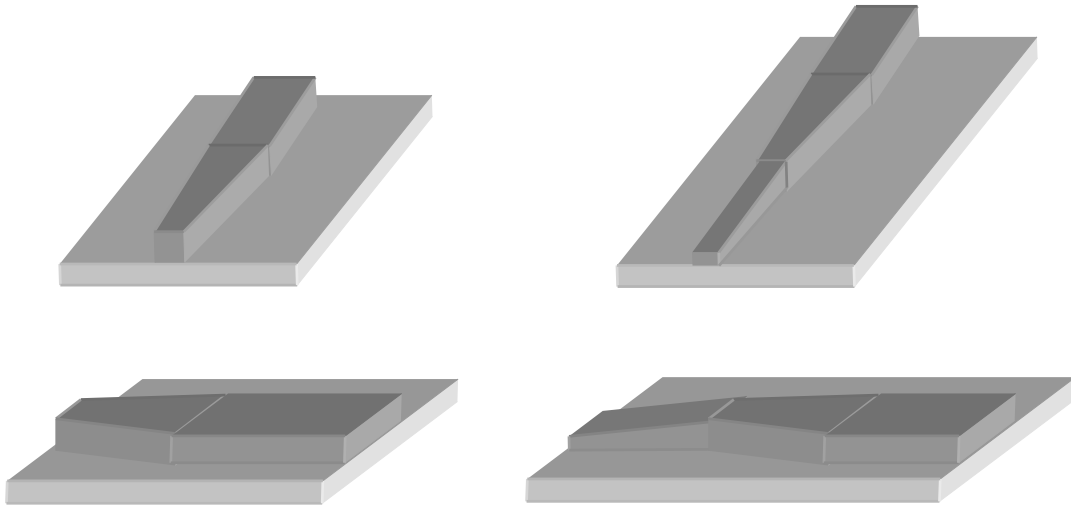
Figure 3.28a. Top and side-view of a horizontal taper.
