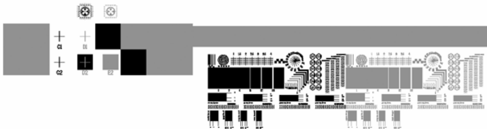
Figure 5.5. Close-up of the alignment bar. This bar contains the alignment markers (left) and several test structures (right).
